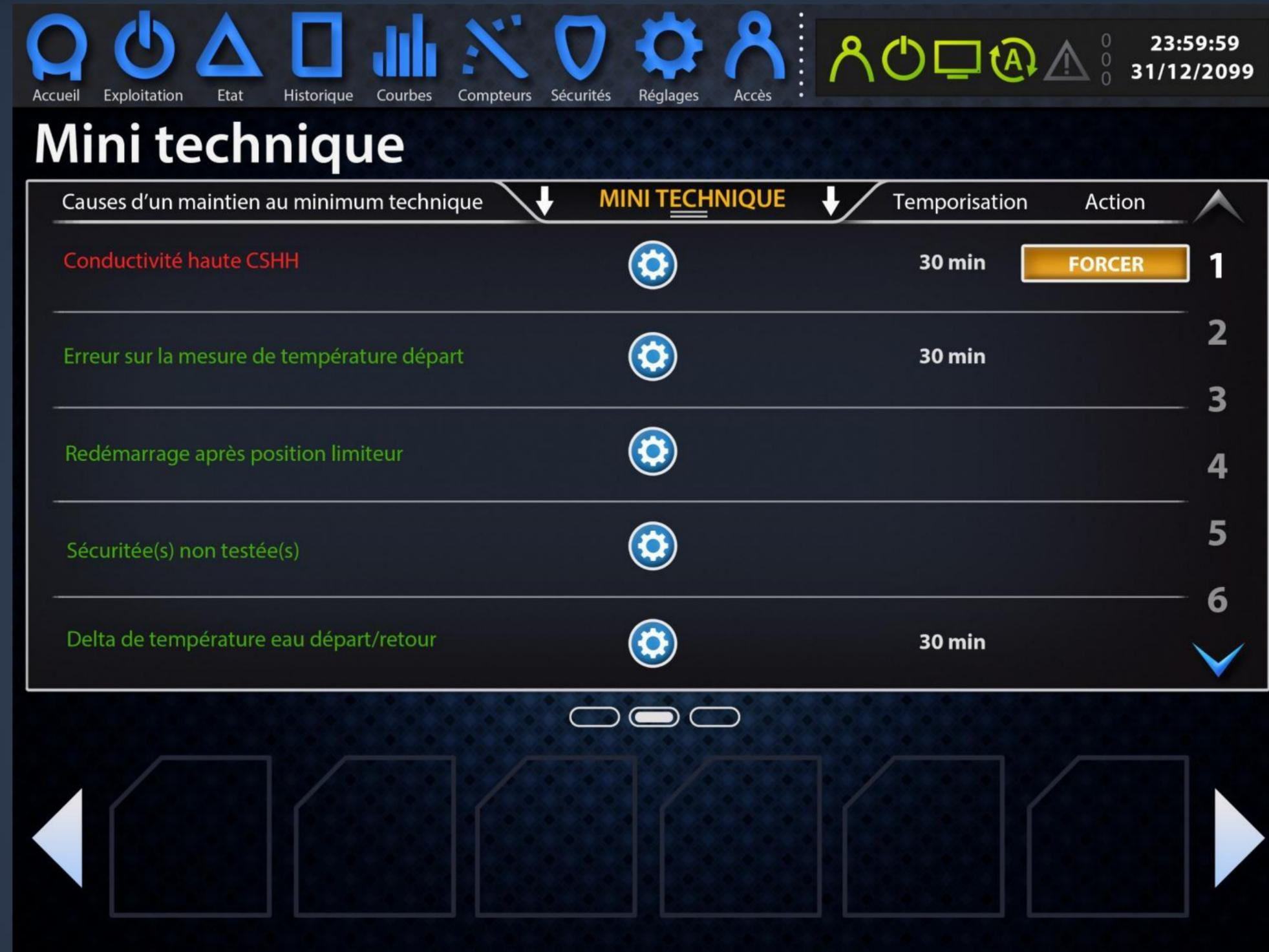
The screenshot displays the 'Mini technique' interface. At the top, there is a navigation bar with icons for Accueil, Exploitation, Etat, Historique, Courbes, Compteurs, Sécurités, Réglages, and Accès. A status bar on the right shows the time 23:59:59 and date 31/12/2099. The main content area is titled 'Mini technique' and contains a table with the following data:
